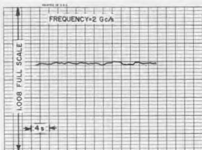
Figure 10. Typical recording of system noise at 2 Gc/s, with Type 1360-B Microwave Oscillator used as signal source. Chart speed was 30 div/min. Note that total excursion over entire 25-second recording is equivalent to VSWR of only 1.0002.
